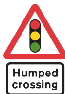
Signal-controlled pedestrian crossing on a road hump
