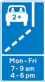
Start of HOV lane (near-side)
