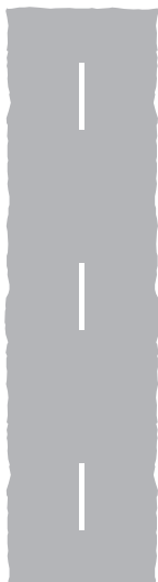
Centre line on a single carriageway road
