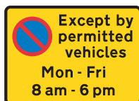
Repeater sign within a loading area
